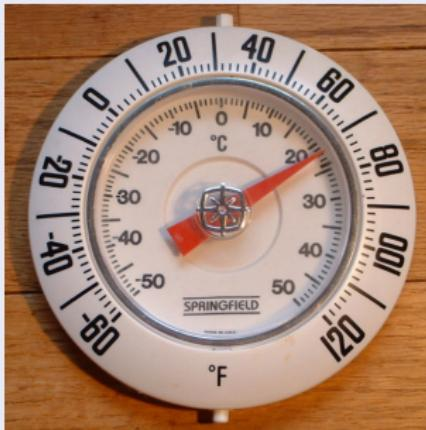
Fig. 2: The thermometer showing the Fahrenheit and Celsius temperatures
